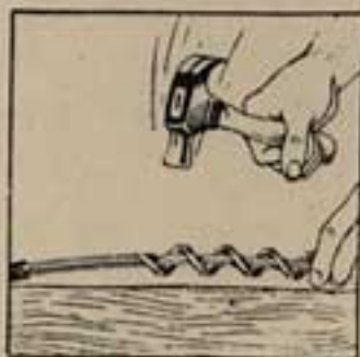
Re-straightening the twist
